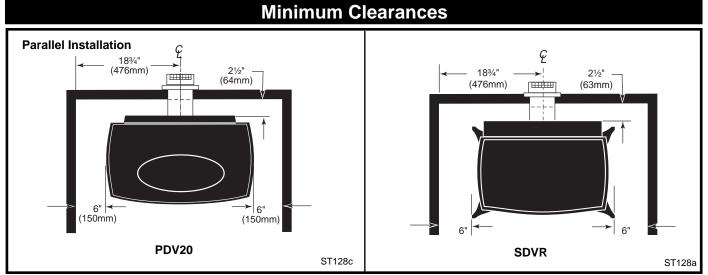
Fig. 3 Parallel installation minimum clearances and flue centerline.
